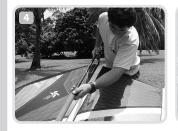
Next, connect the boom to the mast. Clamp the boom on and place the sail down gently. Attach the outhaul, and tension as necessary.
