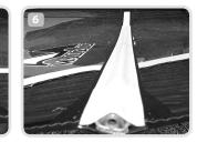
Tension all the battens. Pic. 5 - Visible wrinkles. Pic. 6 - Smooth area after tension applied. Using the small tool supplied with the sail, tension all the battens as necessary to remove all wrinkles, by turning the screw adjuster in a clockwise direction.
